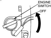
Figure 18. Engine ON/OFF Switch (OFF)
